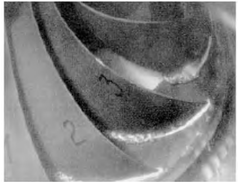
Inlet edge cavitation in Francis turbine
